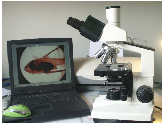
Video Microscope L1180 plugged to Laptop
